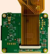
Connect the display ribbon cable to the back of the adapter board (Panel 2)
